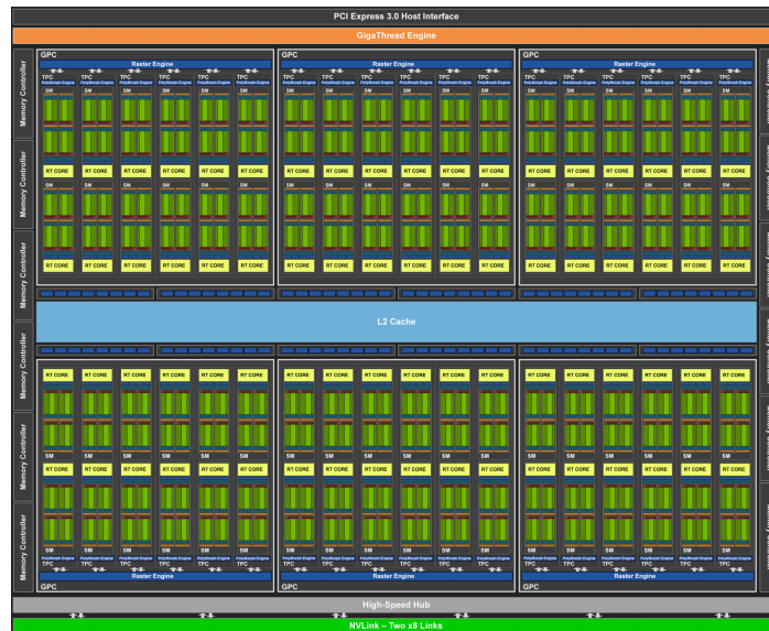
Fig. 12.4.8: NVIDIA Turing architecture (image courtesy of NVIDIA)
